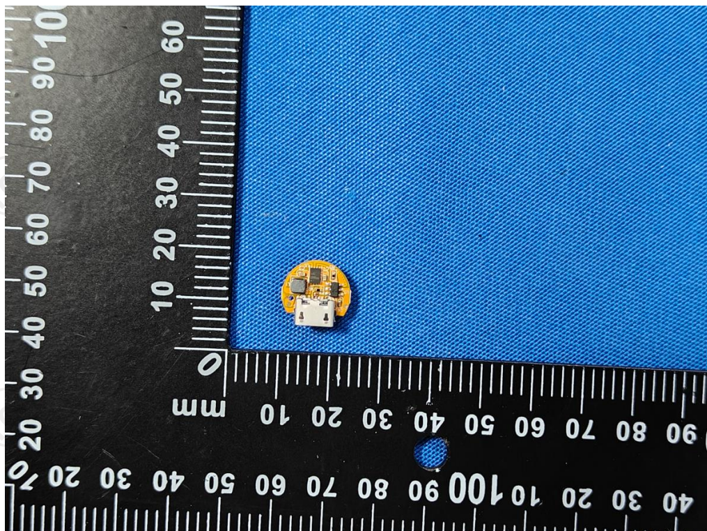
Picture 5. Front view of protection board 图片 5. 保护板前视图
